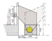
feeding via wall-connected filling chute
